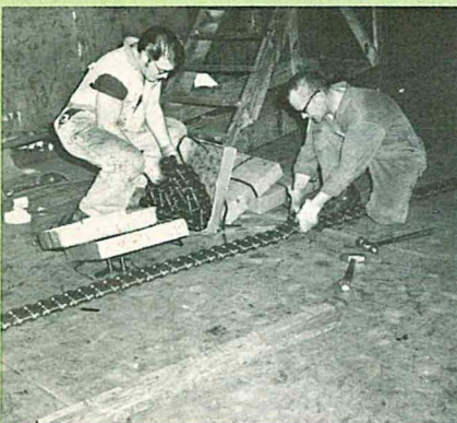
2nd Shift Assemblers Ron Keiser and Dale Bressler unpack and link the chain drive.
